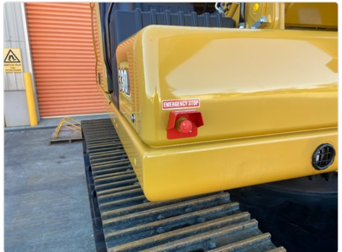
OFF SIDE GROUND LEVEL EMERGENCY SHUTDOWN.
