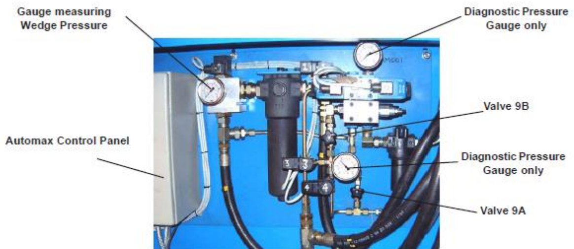
Figure 9g Dumpy Jack Circuit Shut Off Valves
