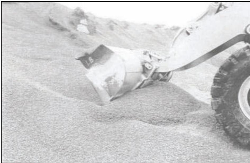
(ii) Level the top of the heap with the power shovel and take sufficient material from near the centre of the levelled heap, ensuring that all material removed is retained, to provide one sample increment from each heap
