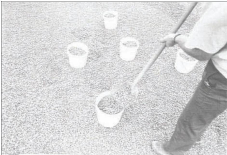
From AS 1141.3.1 Clause 6.2 NOTE: When a single sample increment is used to indicate production quality, the mass of the sample increment should be in accordance with Table 2 (i.e. 5 times the mass of a 5 sample increment mass)
