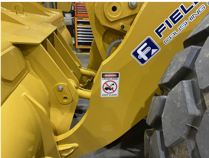
KEEP CLEAR CRUSH ZONE ON LOADER ARMS DECAL
