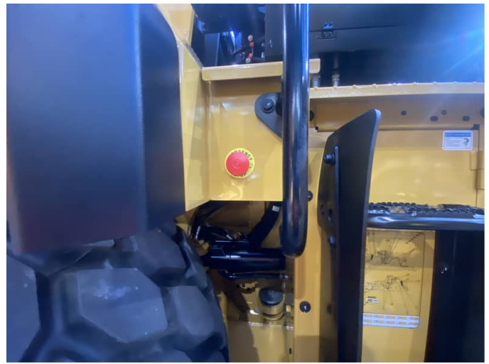
MODIFICATION: OFF SIDE GROUND LEVEL SHUTDOWN
