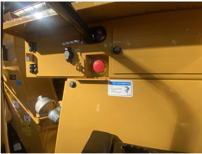
MODIFICATION: ON SIDE GROUND LEVEL SHUTDOWN
