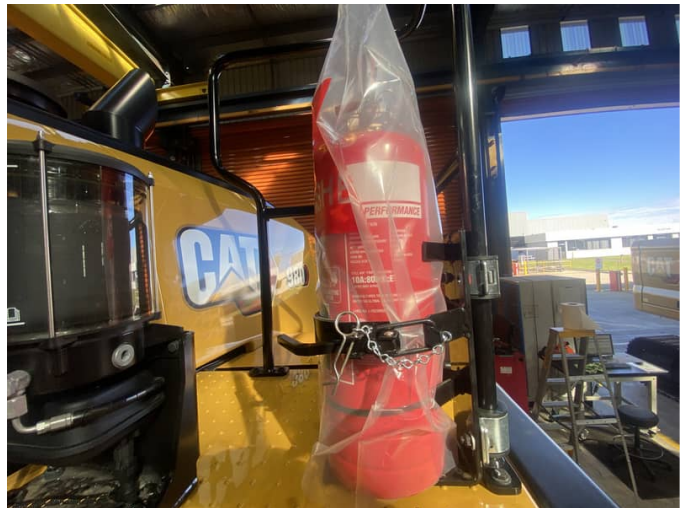
MODIFICATION: 9KG FIRE EXTINGUISHER
