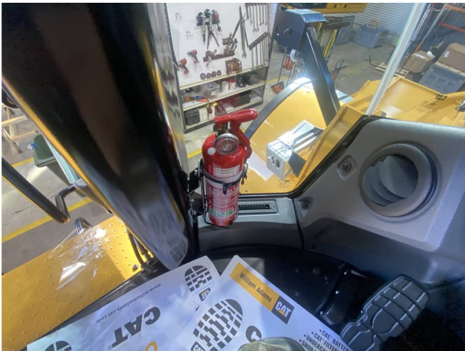
MODIFICATION: 1KG FIRE EXTINGUISHER
